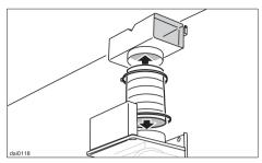
■ Slip the hose clamps over the flex hose onto the diverter and the motor assembly exhaust connection. Once in place, tighten the hose clamps.
